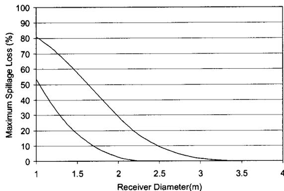
Fig. 7 The yearly maximum spillage loss is shown as a function of the receiver diameter. Lower curve: new heliostat.
