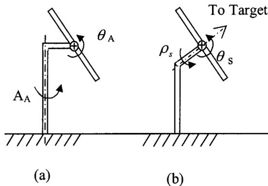
**Fig. 2** The schematic diagram shows the difference between the two kinds of sun tracking methods: (a) azimuth-elevation; (b) spinning-elevation.
