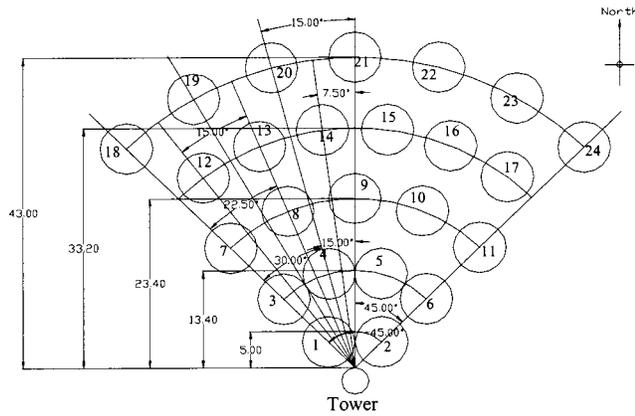
**Fig. 4** The layout shows the heliostat field used for comparison between the two types of heliostat design. The dimensions shown are in meters. The tower height is 20 m. The specifications for each heliostat are given in Table 1.
