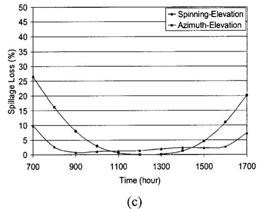
**Fig. 11** The time variation of spillage loss for the entire field diameter is plotted for both sun-tracking methods during June 21. (a) Receiver aperture diameter is 1 m. (b) Aperture diameter 1.2 m. (c) Aperture diameter 1.4 m.
