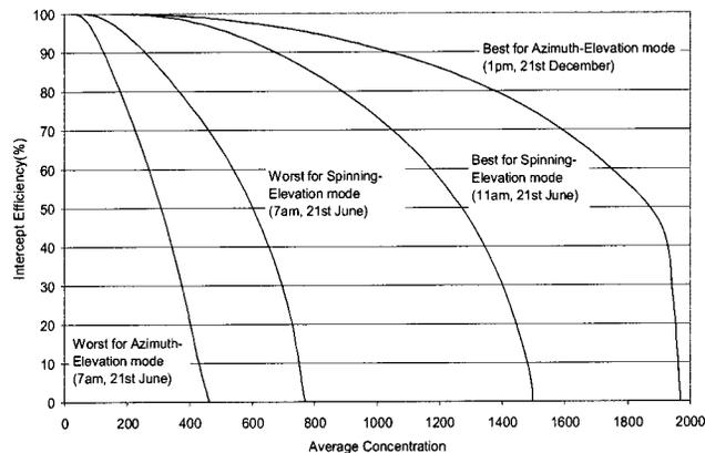
**Fig. 10** The best and worst characteristic curves for both sun-tracking methods are plotted. The characteristic curves for all other times are within the two limits.
