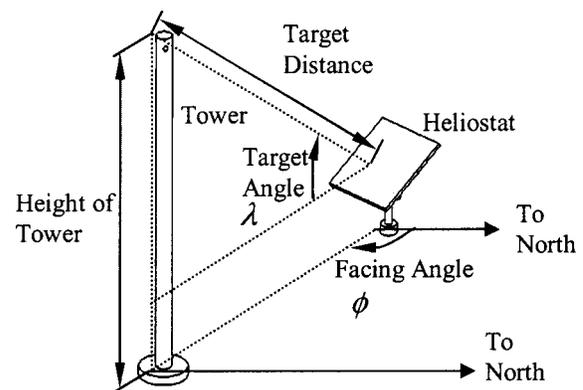
**Fig. 3** The definitions of geometric parameters used in the comparison of heliostats
