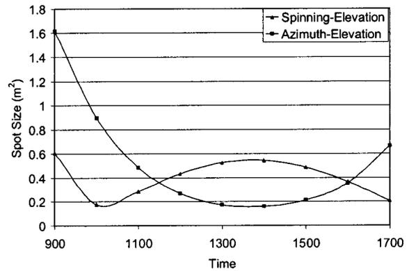
**Fig. 1 Spot size comparison between the spinning-elevation and azimuth-elevation tracking methods for June 21st. The target angle is 41.8 deg, facing angle is 10 deg to the south and the latitude is North 43 deg. Heliostat area is 25 m<sup>2</sup> and the slant range is 30 m.**
